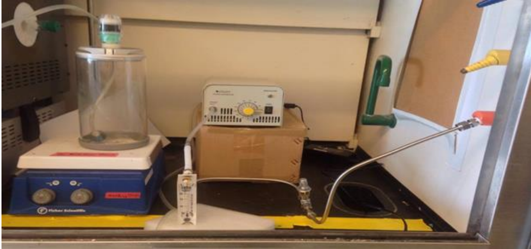
Figure 26. Laboratory-scale set-up of the ozonation system
